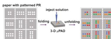
**Fig. 2** Schematic of the 3D paper origami: A paper microfluidic device is fabricated by patterning with photoresist, folded, loaded with aqueous solutions, and unfolded to reveal specific reservoirs filled with the solutions. Figure reprinted with permission from the Journal of the American Chemical Society from Liu and Crooks.<sup>7</sup>
