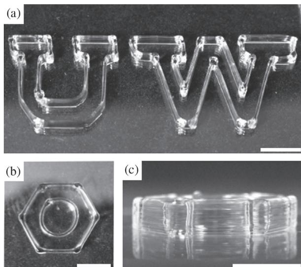
**Figure 5.** 3D printed structures of a 15-layer (a) University of Washington initials and (b, c) benzene ring produced using a 0.41 mm inner diameter nozzle at  $8.0 \text{ mm s}^{-1}$ . This structure was printed with a formulation of polymer **9** at 20 wt% using a pneumatic direct-write 3D printer (scale bars: 1 cm).
